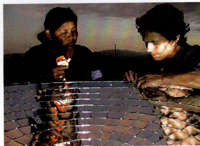
Fabricating the parabolic mirror
